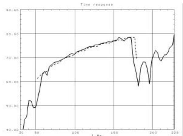
Figure 17. Profiles of swept sine (dashed) and modified order (solid) – Validation of the procedure
