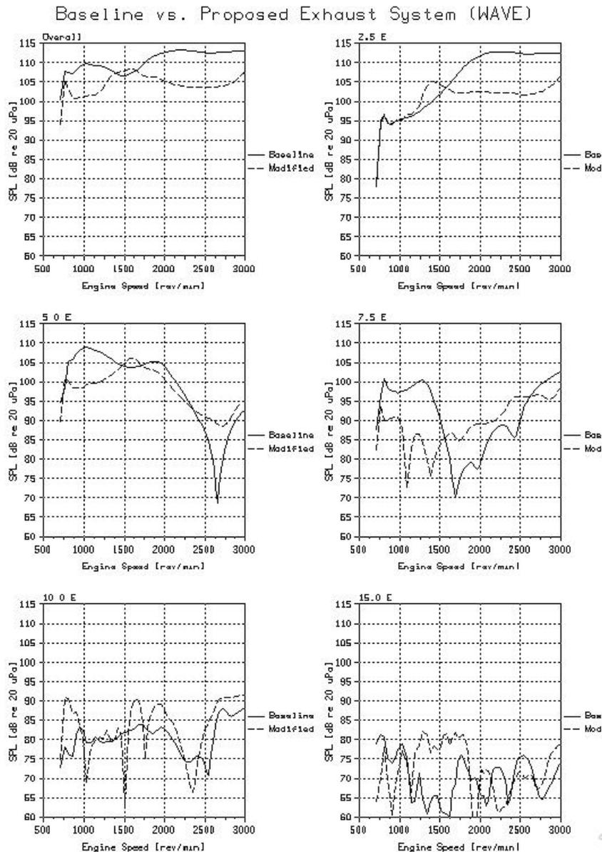
Figure 12. Comparison of predicted tailpipe noise for production system and for proposed modification
