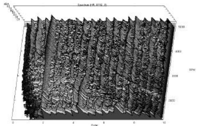
Figure 10. 3D order spectral map for runup in neutral.
