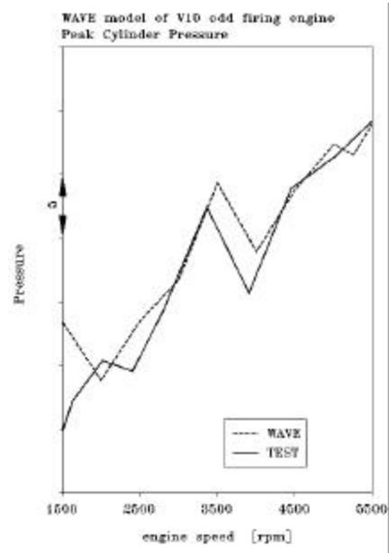
Figure 6. Measured and predicted maximum cylinder pressure
