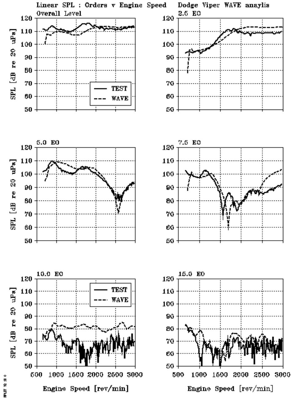
Figure 7. Measured and predicted tailpipe noise: overall and orders 2.5, 5, 7.5, 10 and 15
