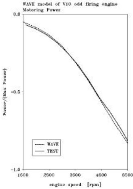
Figure 3. Measured and predicted absorbed engine power under motoring conditions
