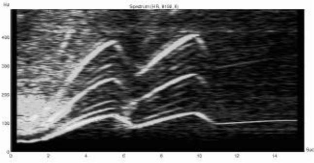
Figure 11. Spectrogram of measured noise of baseline system: Drive-away with moderate throttle opening
