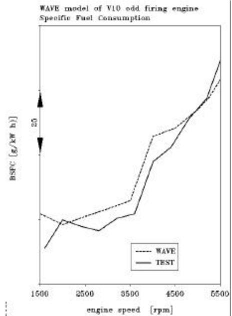
Figure 5. Measured and predicted specific fuel consumption
