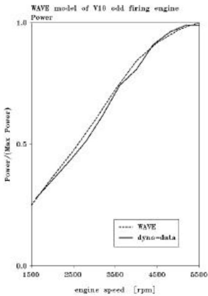
Figure 4. Measured and predicted engine power under full load conditions
