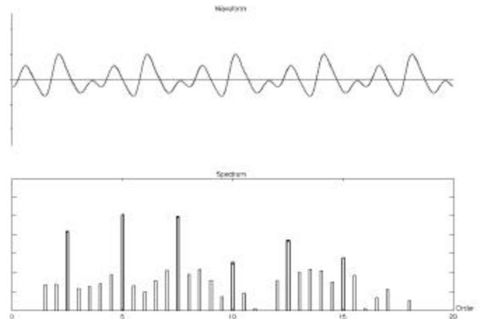
Figure 9. Binaural data at idle for baseline: Average time cycle (top) and corresponding order spectra (bottom).
