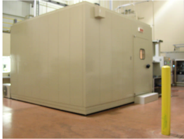
Figure 1. Sound chamber at Michigan Automotive Compressor
