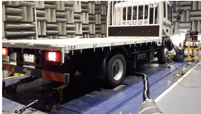
Fig. 9 – Test Setup on the 4 Wheel Drive Chassis Dyno
