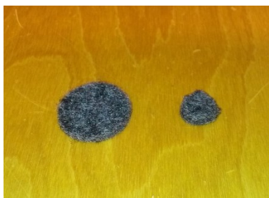
(8a) Image of samples (Left: for Brüel & Kjær 4206 small tube, Right: for HF tube)
