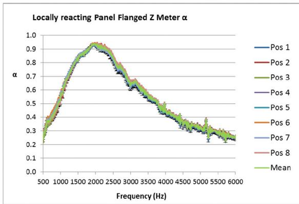
Figure 10. Locally reacting panel. Flanged impedance tube normal incidence sound absorption coefficient,  $\alpha$
