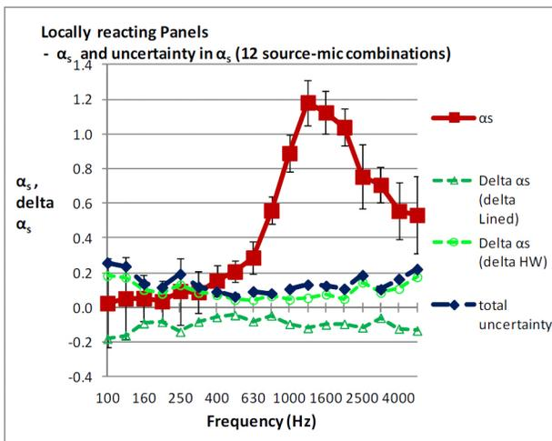
Figure 7. Locally reacting panel Sound Absorption coefficient,  $\alpha_s$ , and uncertainty due to reverberation time standard deviation (12 source/ mic combinations)
