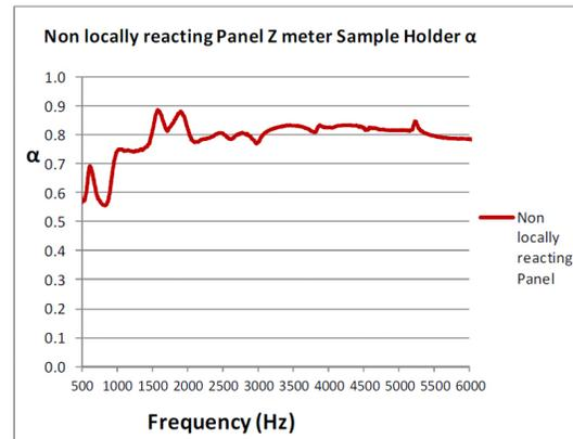
Figure 12. Non-locally reacting panel. Impedance tube sample holder normal incidence sound absorption coefficient,  $\alpha$
