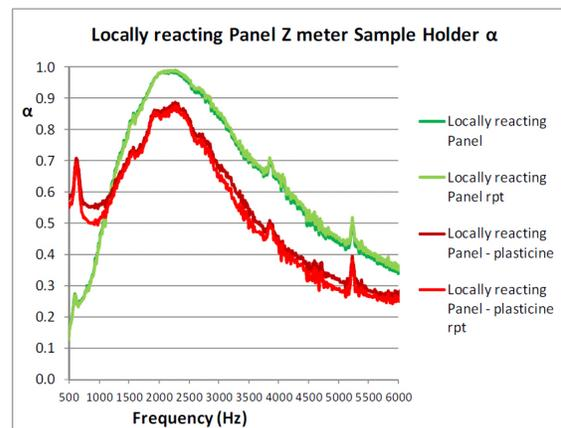
Figure 14. Locally reacting panel. Impedance tube sample holder normal incidence sound absorption coefficient,  $\alpha$
