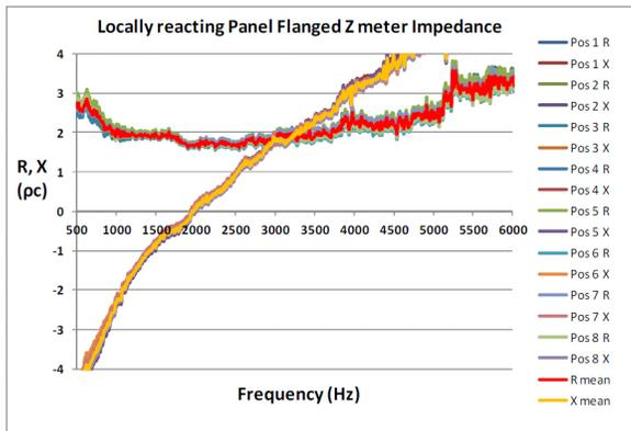
Figure 11. Locally reacting panel. Flanged impedance tube normal incidence impedance
