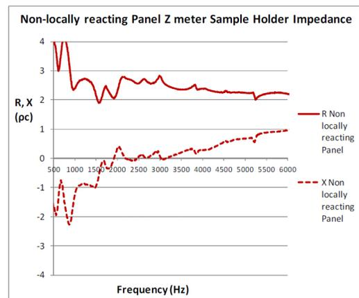
Figure 13. Non-locally reacting panel. Impedance tube sample holder normal incidence impedance
