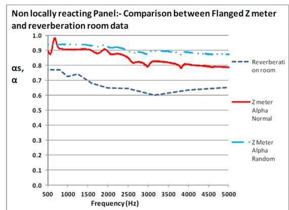
Figure 17. Non-locally reacting panel comparison of reverberation room and flanged impedance tube absorption coefficient measurements
