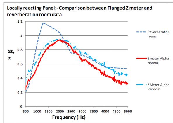
Figure 16. Locally reacting panel comparison of reverberation room and flanged impedance tube absorption coefficient measurements
