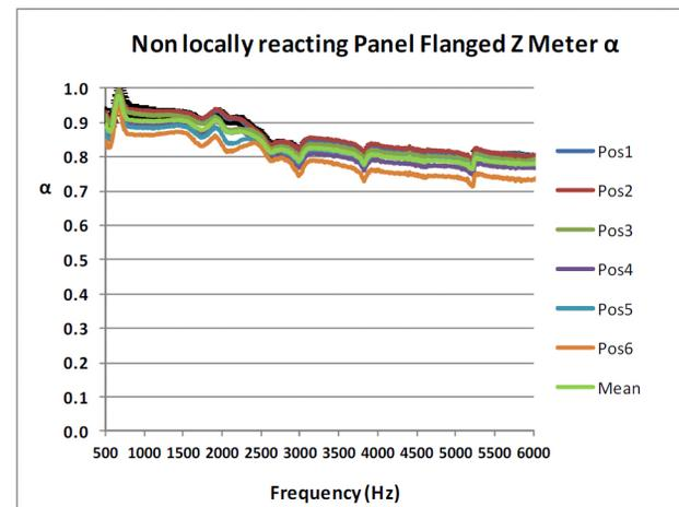
Figure 8. Non-locally reacting panel. Flanged impedance tube normal incidence sound absorption coefficient,  $\alpha$
