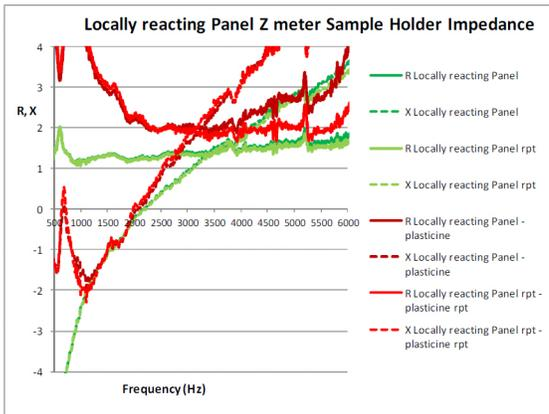
Figure 15. Locally reacting panel. Impedance tube sample holder normal incidence impedance
