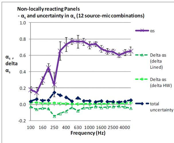
Figure 6. Non-locally reacting panel Sound Absorption coefficient,  $\alpha_s$ , and uncertainty due to reverberation time standard deviation (12 source/ mic combinations)
