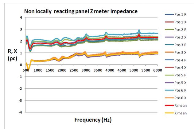
Figure 9. Non-locally reacting panel. Flanged impedance tube normal incidence impedance
