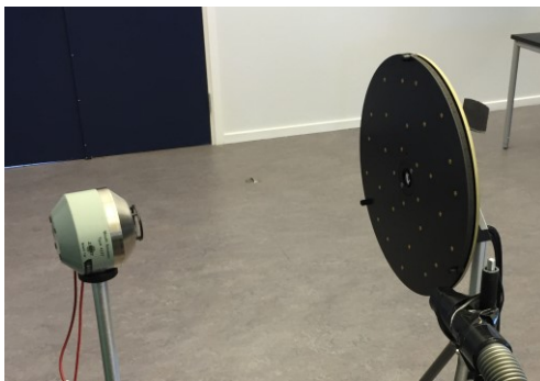
Figure 12 – Picture of the setup with array (right), source (left) and flow-beam hose (bottom right).
