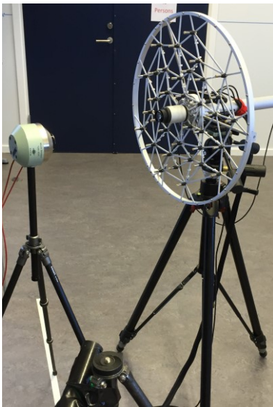
Figure 5 – Picture of the setup with array (right), source (left) and flow-outlet nozzle (bottom).
