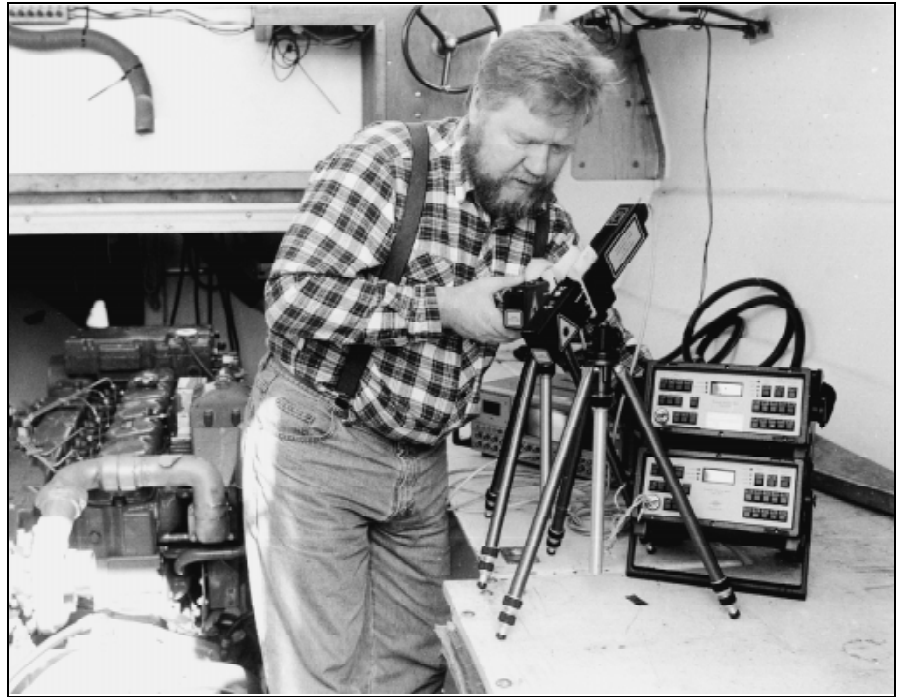
Two Torsional Vibration Meters Type 2523 being prepared for a marine application. The operating principle ensures that the instrument can be employed even in severe environments with maintained confidence in the results
