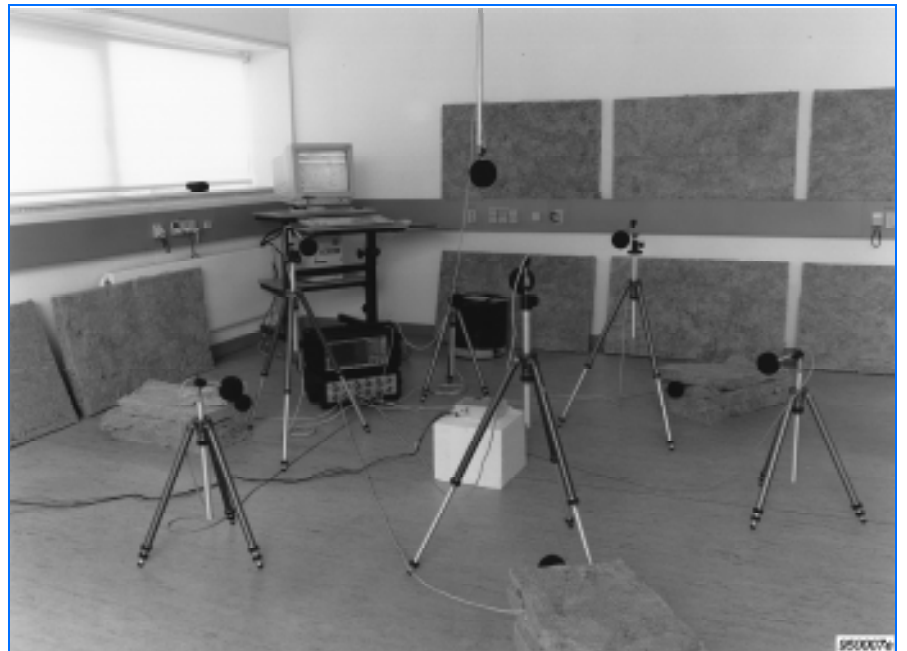
Fig.4 Sound power determination in an office according to ISO 3744. With the reference sound source Type 4204, which can be seen behind the tape streamer, the acoustic properties of the room can be determined. To obtain sufficient absorption, absorption material had to be installed
