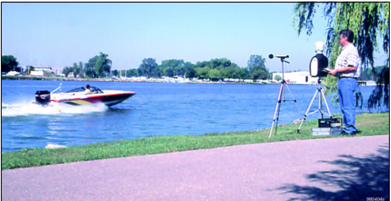
Fig. 4 Making a pass-by measurement with the Head and Torso Simulator on the shoreline and a boat passing by at full throttle
