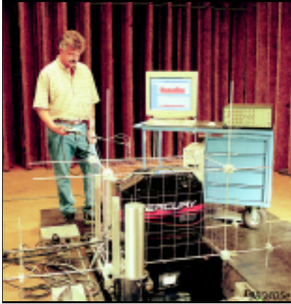
Fig. 3 At Mercury Marine PULSE is used daily. On the right, PULSE shown being used for modal testing, and below for sound intensity measurements
