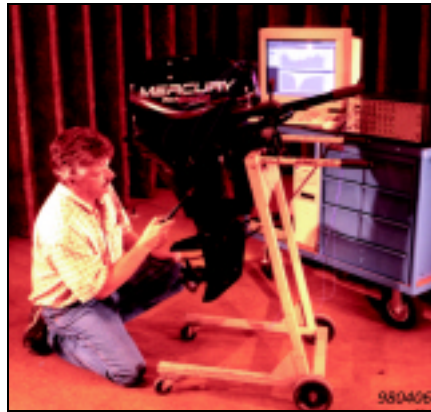
Fig. 3 At Mercury Marine PULSE is used daily. On the right, PULSE shown being used for modal testing, and below for sound intensity measurements
