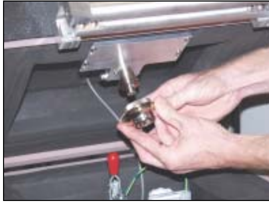
Fig. 3 A Type 4185 Ear Simulator for Telephonometry is attached to a Type 4192 Microphone in one of the test boxes
