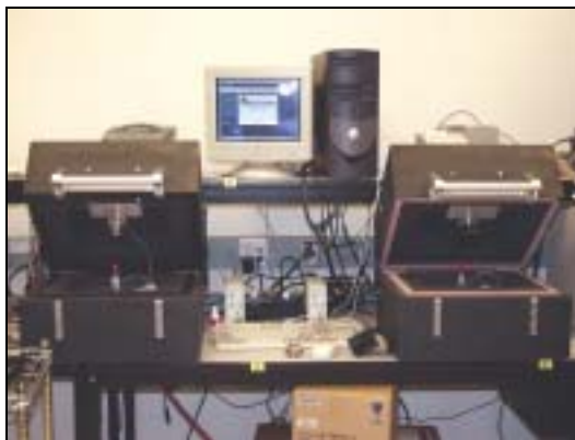
Fig. 2 A testing station showing two test boxes, power amplifiers and a power supply
