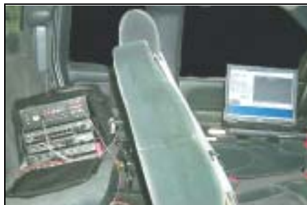
Fig. 7 In-vehicle testing – Link's 3501 system installed in a truck cab
