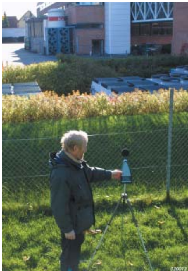
Fig. 3 Measuring fan noise at the fence
