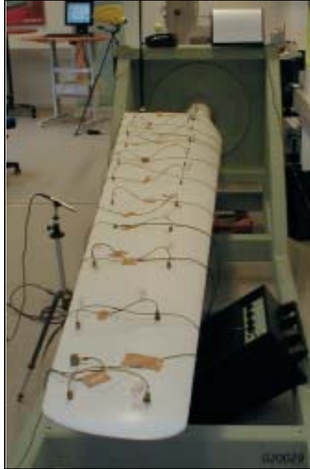
Fig. 1 Wind-turbine wing with acoustic excitation. Observe loudspeaker beneath the wing
