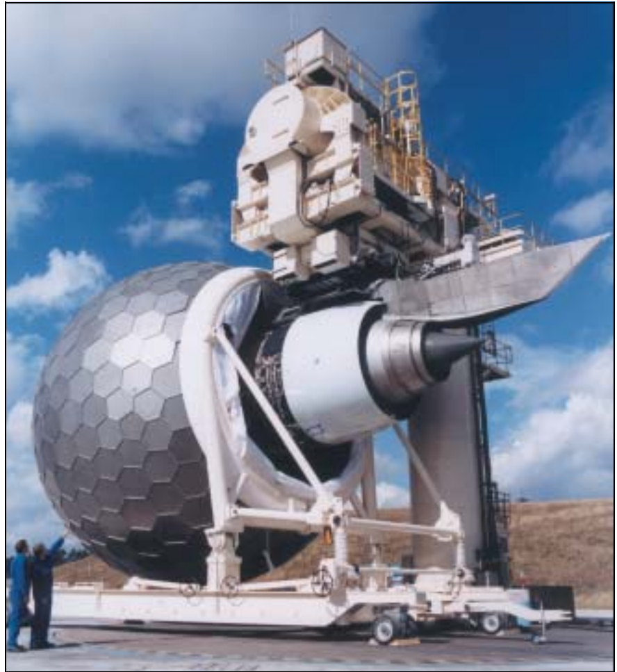
Fig. 1 A Rolls-Royce Trent 500 installed on the Noise Measurement Test Bed at Hucknall. The Turbulence Control Screen is mounted on its own trailer.
