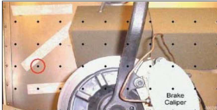
Fig. 1 Measurement area with dots indicating array microphone positions
