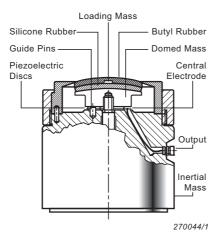
The inertial mass is shown in cross-section in Fig. 1. It weighs 3.5 kg, is machined from ECO BRASS® and is nickel-plated.
