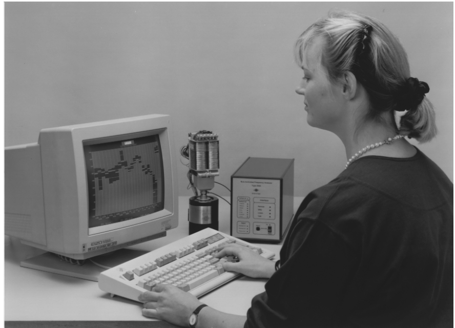
Fig.2 Using the 2140/WH2857 with the QCMASK program to measure the mechanical power of a small motor
