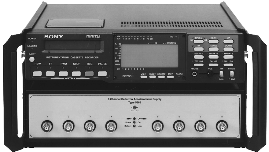
Fig. 2 Type 5963 and DAT recorder as one package, the Type 9658
