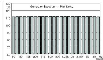
The built-in generator can supply pink noise or white noise in the bandwidth used for the measurement. The signal is switched on and off automatically in accordance with the performed measurement.
