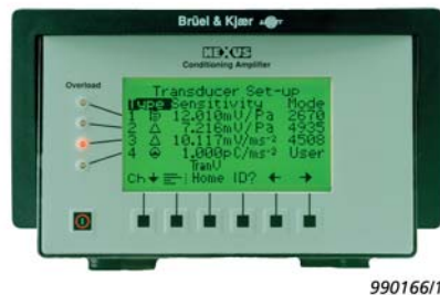
Fig. 8 Transducer setup. The sensitivity and mode fields have been automatically read from the IEEE 1451.4 compatible transducers
