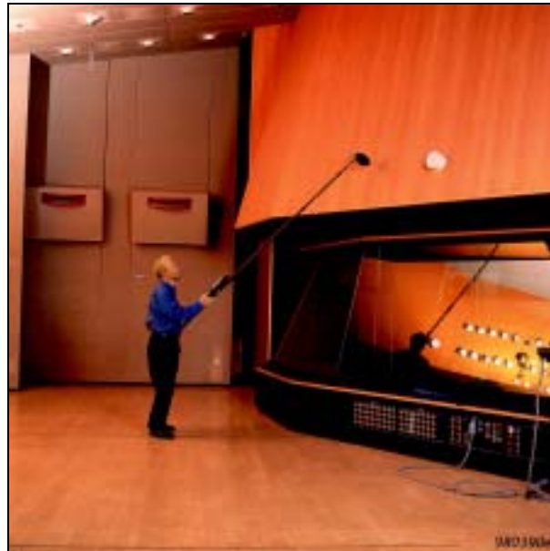
Fig. 10 Mapping the sound reduction to find leakages between studio and control room
