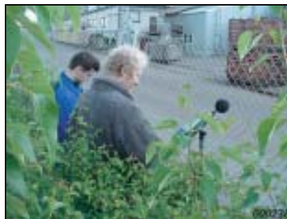
Fig. 4 Using FFT to evaluate the tonal content of noise at the boundary of an industrial plant
