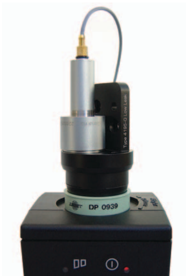
Fig. 3 The coupler mounted with the Standard Adapter Ring for 'on-the-line' sensitivity verification, using Sound Calibrator Type 4231 with Calibration Adapter DP-0939
