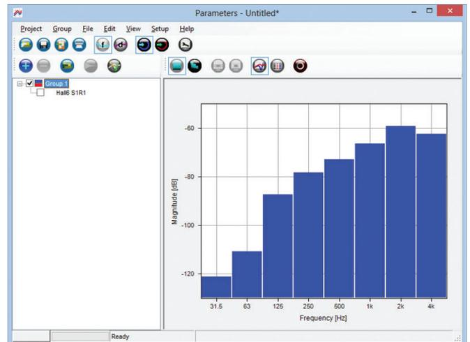
Fig. 22 Parameter graph showing D<sub>50</sub> average and standard deviation over four receiver positions
