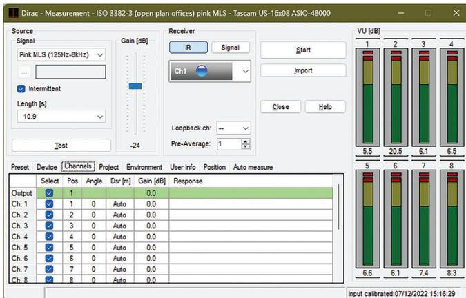
Longer excitation times can be used to suppress background noise. Each doubling of excitation time results in a 3 dB reduction in background noise. In this case, a reverberation time of around 1 second is expected, and an excitation time of 10.9 seconds will improve the impulse response-to-noise ratio (INR) by over 10 dB compared to traditional measurement methods.
