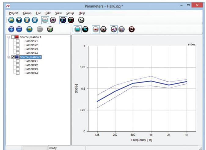
Fig. 23 Parameter graph showing  $D_{50}$  average over four receiver positions, for two different source positions
