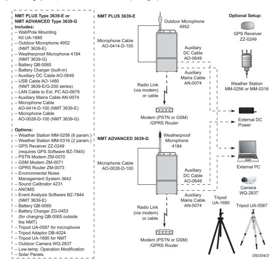
The NMT is controlled remotely by Environmental Noise Management Software Type 7843 (see BP 2100), ANOMS airport noise monitoring software or Noise Monitoring Software Type 7802 (see BP 1573), allowing remote setup, data and system status viewing, data download and analysis. An option allows the user or system integrator to implement control by third party software, through the documented instruction set included with the relevant configurations.
