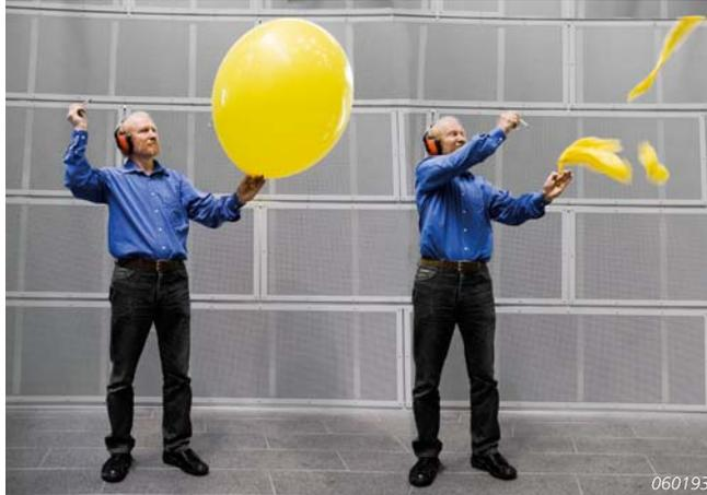
With Impulsive Excitation, all you need to carry is Type 2250-F, a tripod and a balloon (or other impulsive source, such as a starting pistol). After you pop the balloon, Type 2250-F will start measuring, analyse the decay and present the RT as well as the decay curves for all frequency bands.
