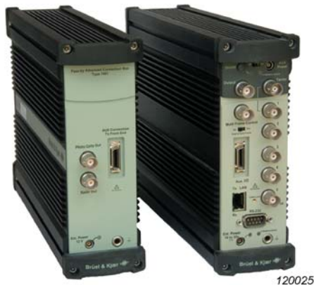
Fig. 3 The Pass-by Ground Station consists of a 5-channel data acquisition unit with BNC connectors, PULSE Multi-analyzer Type 3560-B, and Advanced Connection Box Type 7451
