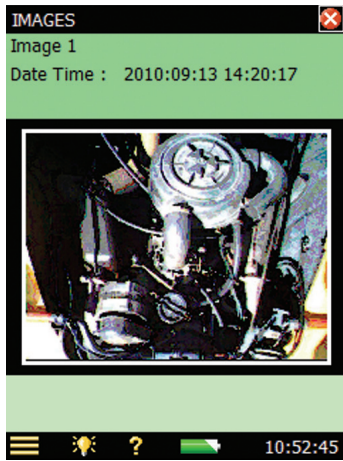
Fig. 6 Use the built-in camera in Type 2270 to photograph the test device
