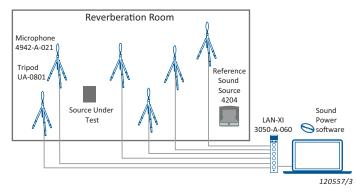
Setup with high-frequency sound power determination 1/2" Diffuse-field TEDS Microphone Type 4942-A-021 is recommended for making measurements using Type 7888 because of its flat frequency response over the desired frequency range. The microphone can be used with Input Module LAN-XI 51.2 kHz Type 3050 which includes Front Panel UA-2100.
