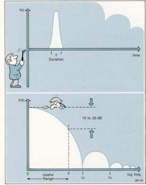
'This analogy is not strictly correct since the tip does not filter out energy: it determines the frequency range where the available energy is concentrated. *Impact hammers* are constructed by adding a force transducer to a hammer, and adding a stiffness-controlling element to the end of the transducer.
