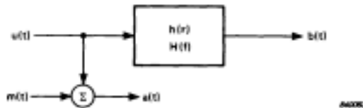
Fig. 16. Ideal system with extraneous noise in measured input signal a(t)
