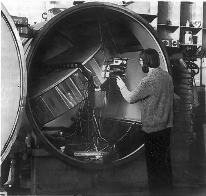
Fig. 6. An experiment with the Wind Wheel in a vacuum chamber for measuring the air pressure correction
