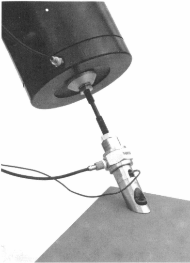
Fig. 2. Application of transducer head using an attached exciter
