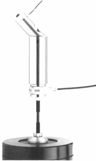
Fig. 7. Checking the dynamic characteristics of the transducer head by mass ratio calibration
