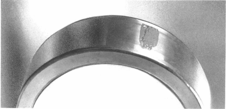
Fig. 20. A roller bearing with a fault, taken out of operation more than five months after the first indication of a fault
