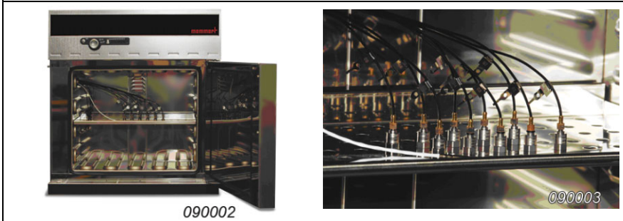
Fig. 3. Oven with accelerometers (left) and close-up of accelerometers (right)
