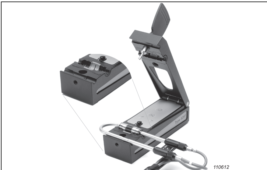
Fig. 2. The final calibrator. The probe is a \frac{1}{2} " probe with a 12 mm spacer. The slit with the sound source is seen in the middle of the coupler cavity
