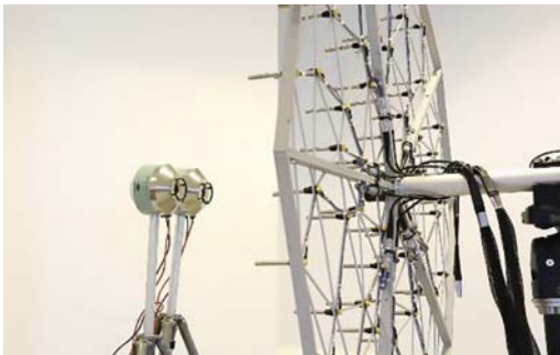
Fig. 12. 60-channel array at 36 cm distance from two Brüel & Kjær mouth simulators, Type 4227
