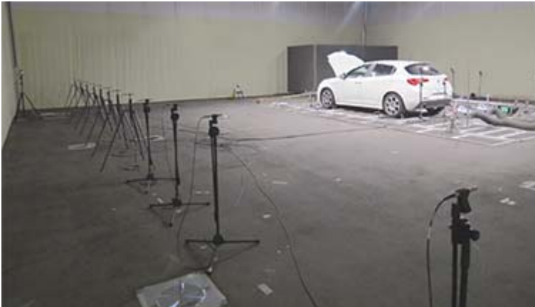
Fig. 8. Single-side indoor pass-by measurement set-up with additional indicator microphones for contribution analysis
