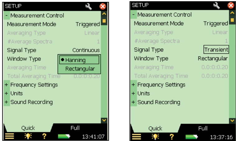
Fig. 4.4 Left: Selecting Window Type from the Setup Page Right: Selecting signal type from the Setup Page
