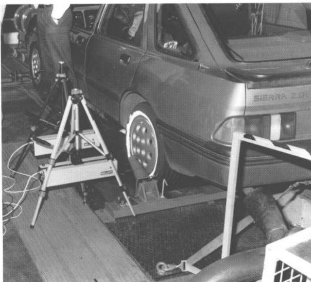
Fig. 13. Measuring differential vibration on a tyre as it spins (photograph courtesy of The Ford Motor Company (UK) Ltd.)
