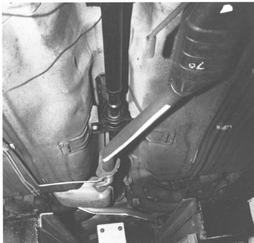
Fig.2 Retroreflective tape attached to the hot exhaust system of a car (photograph courtesy of The Ford Motor Company (UK) Ltd.)
