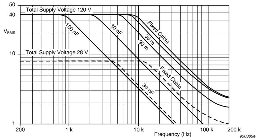
Fig. 2 Upper distortion limit (3%) as a function of preamplifier output voltage and frequency for various capacitive loads. The full-drawn curves are valid for a preamplifier powered with 120 VDC ( $\pm 60$  VDC) and the dotted curves are for 28 VDC ( $\pm 14$  VDC)
