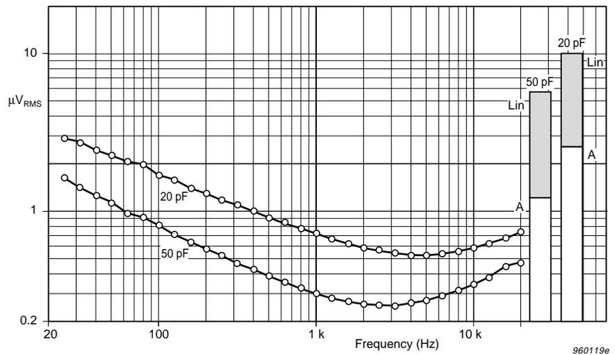
Fig. 3 Typical noise frequency spectra in  $\mu$ V measured with 20 pF and 50 pF microphone capacities. The spectra are measured in  $1/3$ -octave bands with levels at centre frequencies indicated by circles. The bar graphs represent broad-band (22.4 Hz to 300 kHz) and A-weighted noise levels for both microphone capacities
