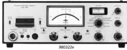
Fig. 4. Reciprocity Calibration Apparatus Type 4143. Manual instrument for reciprocity calibration of microphones which is widely used today
