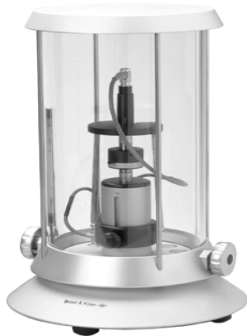
Fig. 9. The sound isolating measurement chamber of Type 9699. The chamber may be pressurized to any value between that of sea level and Mexico City
