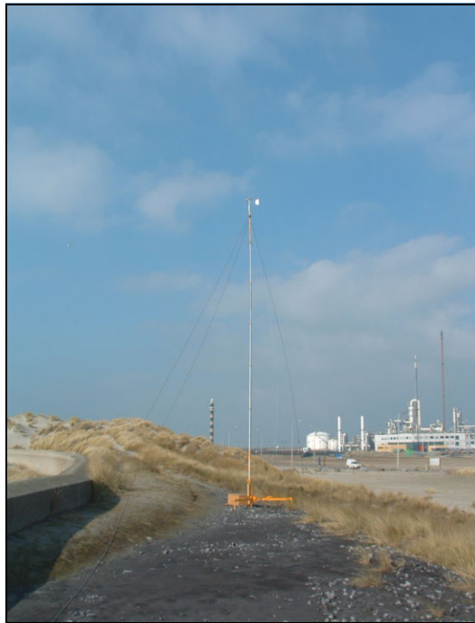
Fig. 3 The relationship between noise measurements and wind speed is determined using the wind speed and direction measurements at a height of 10 m
