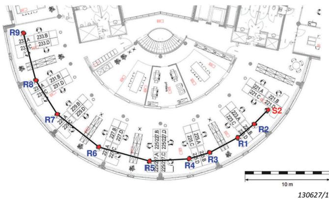
The loudspeaker source is positioned at one of the workstations (S2) and a sound level meter (SLM) is moved in turn to each measurement position (R1 – R9). DIRAC, running on a laptop, switches on the speaker test signal and instantly calculates the speech intelligibility indices from the sound level meter microphone signal. Multiple (wireless) sound level meters can significantly speed up the measurement process.
