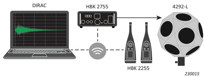
If the PC is far from the source or the microphones, a wireless setup becomes useful. Fig. 4 shows a wireless setup where the PC, sound device (HBK 2755) and one or more sound level meters communicate via Wi-Fi®.
