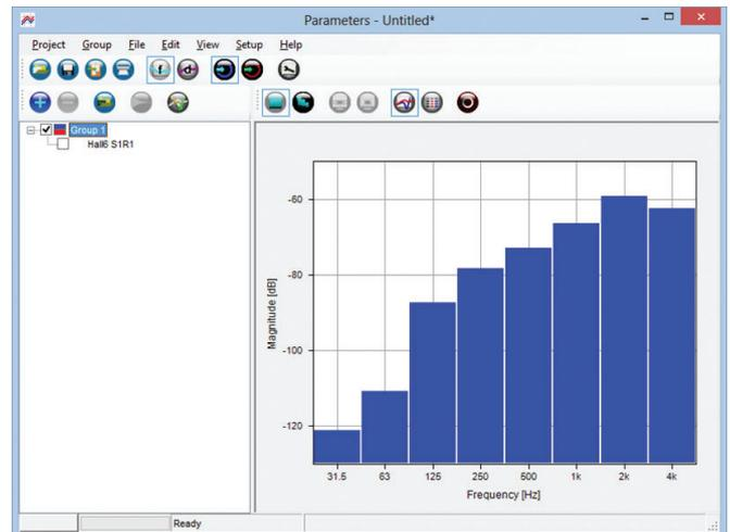
Fig. 22 Parameter graph showing  $D_{50}$  average and standard deviation over four receiver positions
