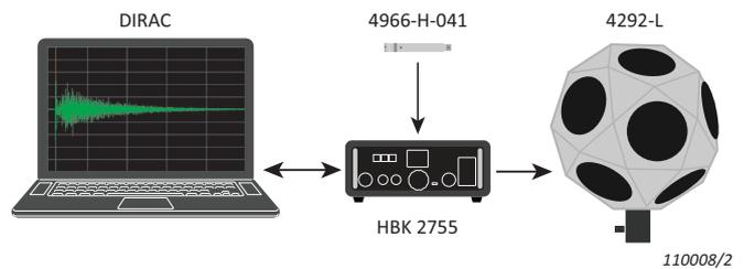
Fig. 2 illustrates the typical use of DIRAC to measure reverberation time and speech intelligibility in an open-plan office. The system components are shown in Fig. 3 and include HBK 2755 Smart Power Amplifier which can be used as a sound device (see The Sound Device on page 4).
