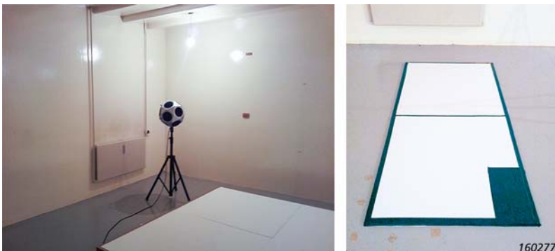
Fig. 3. Non-locally reacting (left), and locally reacting (right), test panels
