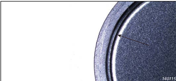
Fig. 4 Magnification of laser-welded diaphragm
