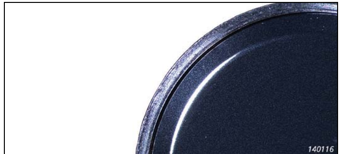
Fig. 5 Magnification of press-fitted diaphragm
