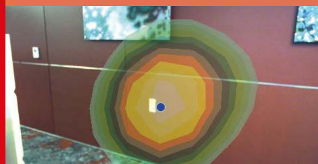
Hot spot found – in this case an electrical outlet
