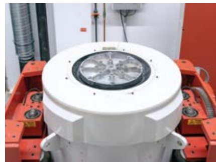
The LDS V8 shaker system with its new hydrostatic bearing table
