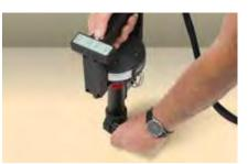
Portable Impedance Meter Type 9737 is a user-friendly kit for quick, non-destructive acoustic material testing
