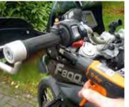
To ensure the reproducibility of the measurements, the accelerometers were mounted with cable straps and a tool to tighten the straps with always the same force
