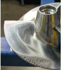
Along with noise, when a steam bubble implodes, it creates a micro-jet that, over time, can result in considerable damage to materials in the immediate vicinity
