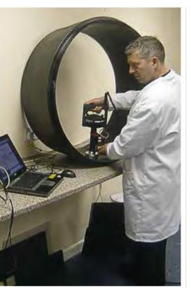
Impedance testing of a GKN Aerospace zero splice acoustic panel
