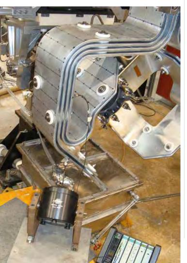
shakers – approximately 200 points were selected from an existing finite element analysis (FEA) wireframe model to create the experimental modal analysis (EMA) model.
