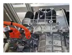
Transmission in a test stand
