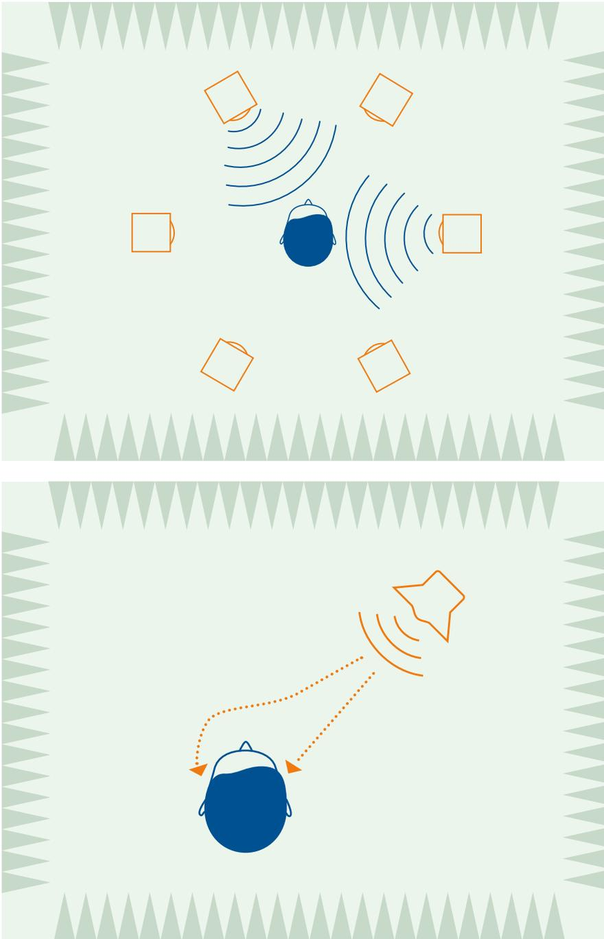
Fig. 3: Measurement of the HRTF for a source at a specific angle
