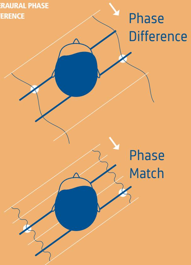
Fig. 1b: While usually the ears will sense a phase difference (top), depending on frequency and angle of incident they may detect a false phase match (bottom)
