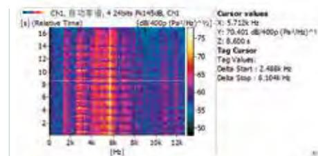
We carried out an FFT vs Time analysis to obtain an RMS spectral density spectrogram
