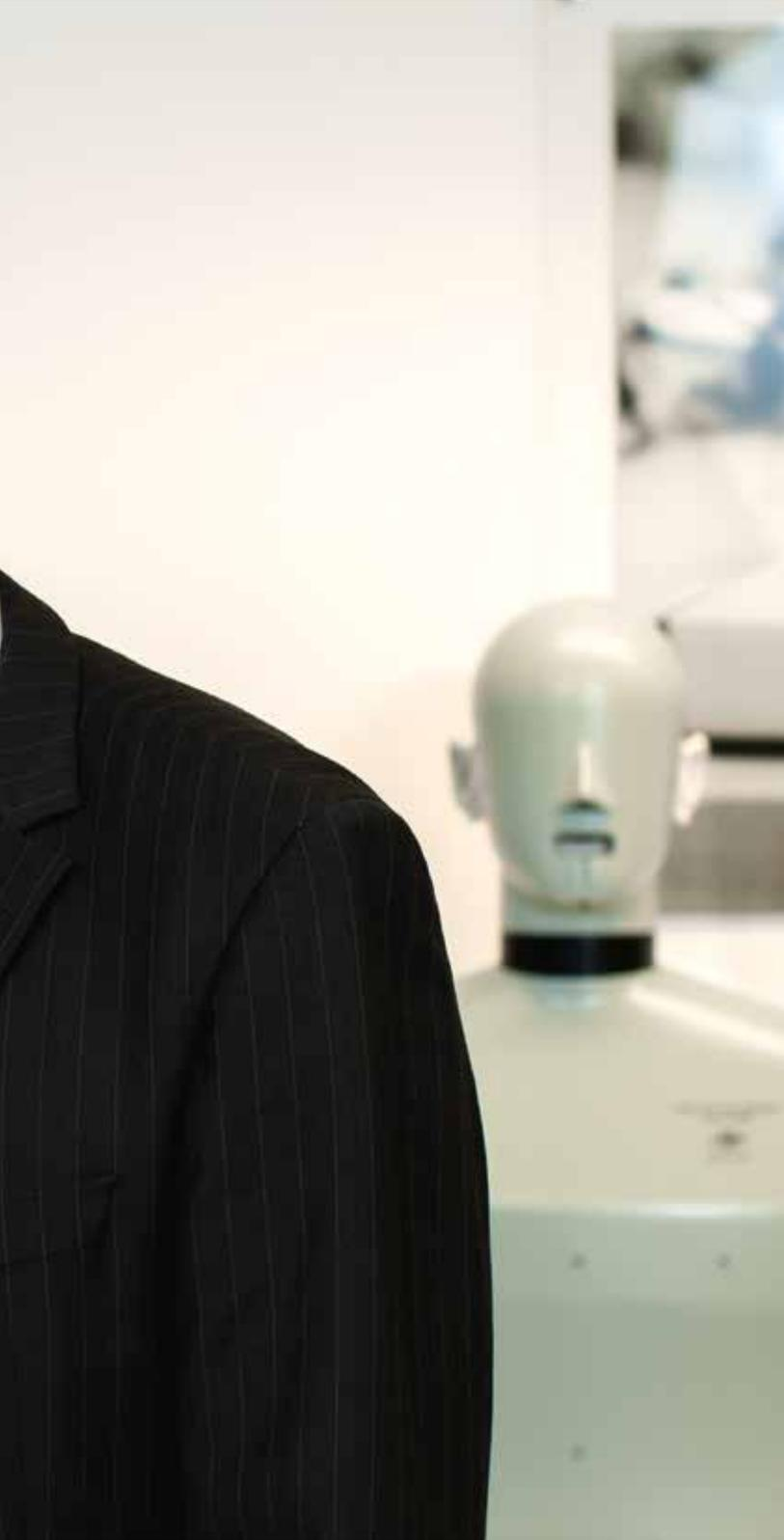
Walk into any acoustic laboratory and you will inevitably see a device that stands out because, unlike most of the boxy instruments in the room, it has the shape of a human head and torso. No surprise then that it's called a head and torso simulator, or HATS for short.
