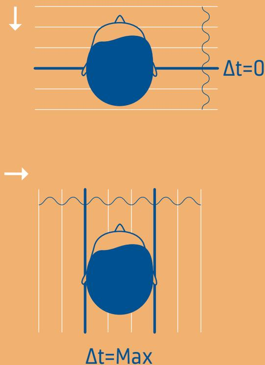
Fig. 1a: With sound coming from the front, the interaural time difference is zero (top). Coming from the side, with a head size of about 20 cm and a sound speed of 340 m/s, the maximum time difference is 0.58 ms
