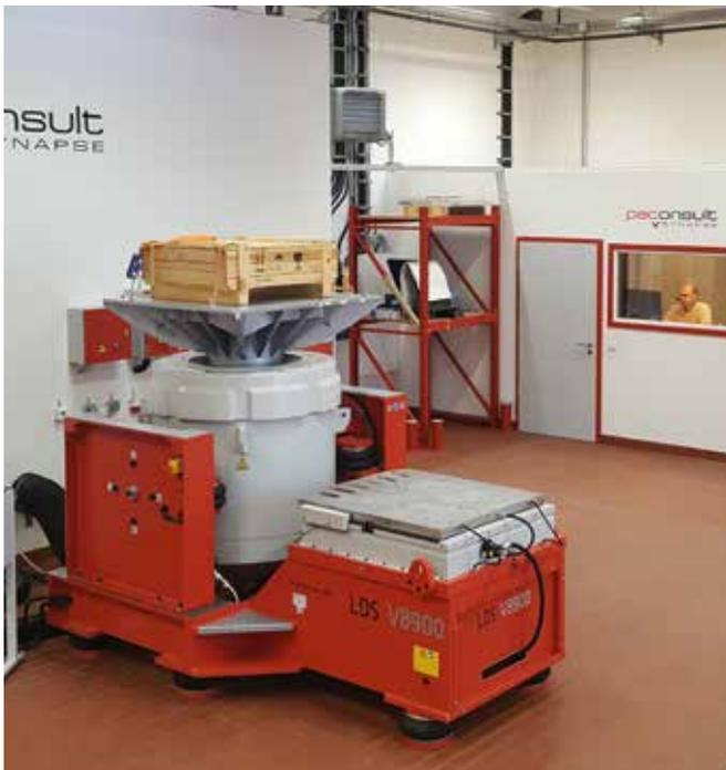
The integrated hydrostatic bearing, which is integral to the high overturning moment restraint, also provides other benefits. This stability makes it easy to work with the shaker and quickly switch out various head expanders and attachments, such as driver bars that connect the shaker and slip table together in the horizontal position so that payloads with large footprints, or standing surfaces, can be tested.
