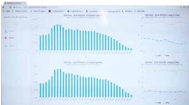
Overview of the time-updated acoustic levels and spectra via the Web-based MONICA common operational picture (COP)
