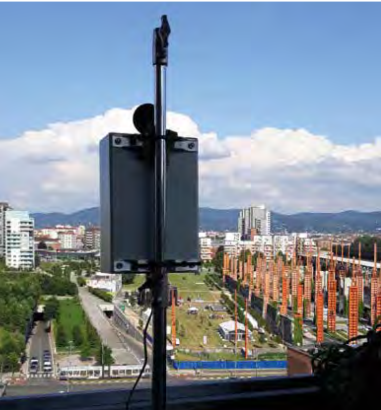
Five sound level meters were placed in the most exposed private residences outside the festival grounds to monitor the music's impact on non-concertgoers nearby
