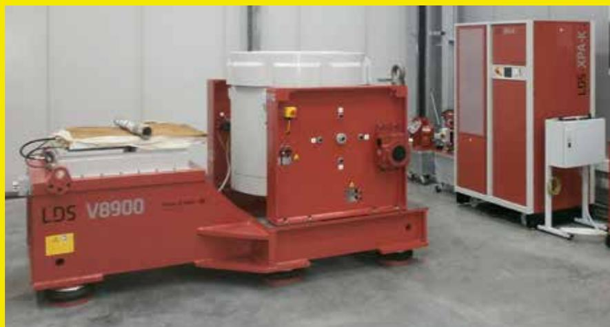
was chosen due to its outstanding shock performance, strong armature hydrostatic guidance and a unique power-saving profile available on the XPA-K range of amplifiers. In addition, a maintenance contract ensures high-level and continued
