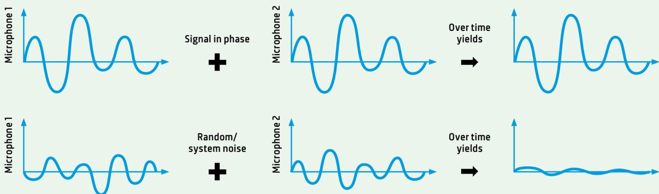
A graphical representation of the correlation process for microphone signals. Because the microphones are so close, external noise will be functionally simultaneous and, therefore, in phase (correlated), and random/system noise will be significantly out of phase and, over time, average to zero.
