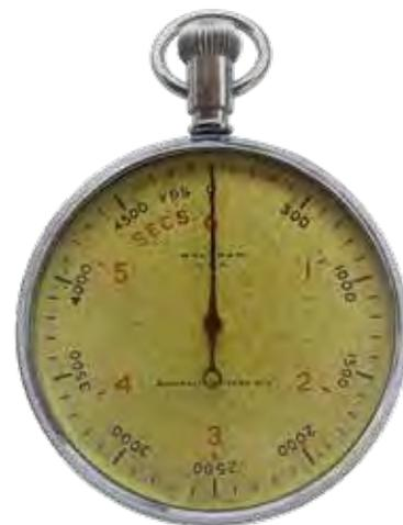
This is a Waltham Sonar chronometer used in WWII. The chronometer utilizes sonar waves to measure the distance between a submarine and another boat.
